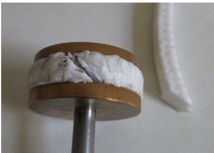
The piston fitted with new square PTFE braided rope gland packing ready for squeezing back into the cylinder. Note the ends are cut at about 45 degrees to make an overlapping scarf joint.
