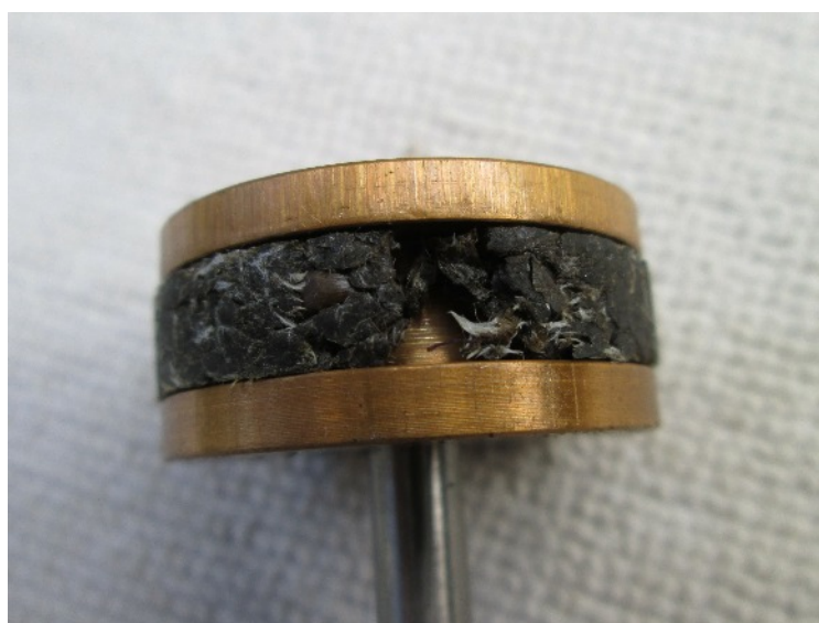
The 3/16 inch square graphited yarn had spread in the 1/4 inch wide piston groove and the joint opened up by about 1/8 inch. Not a good way to make a seal.
