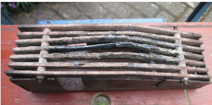
The original grate was severely burnt and somewhat distorted after more than 90 hours running in my ownership.
