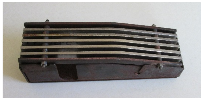
The new grate ready for another 100 hours running? Note the gap in the side of the ash-pan where the rear axle passes through!
