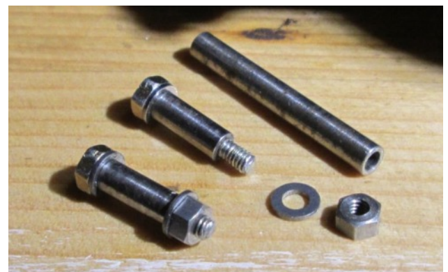
My new pin consisting of a small hollow cylinder of \frac{1}{8} " silver steel screwed onto an 8BA hex head screw.
