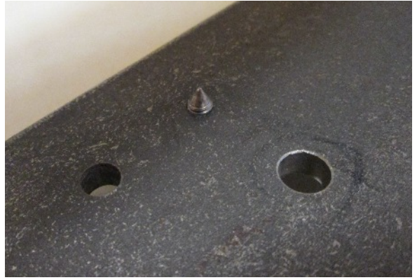
The little cone seen here supports the axle by locating in a centre drill hole in the axle end. The larger of the two holes locates the crank pin, the smaller one is redundant.
