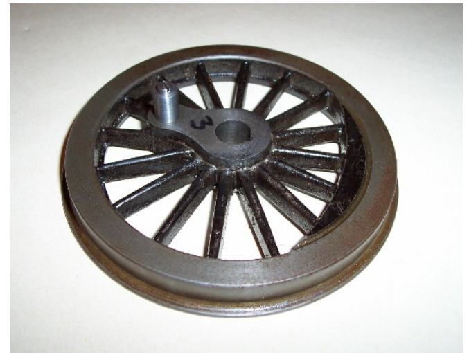
This wheel has a sleeve on the crank pin to fit the larger holes in the jig side plates.
