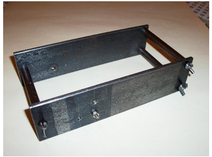
This is my wheel quartering jig complete with scribe marks from marking out! The 2BA nut you can see locks the axle support cone in position.
