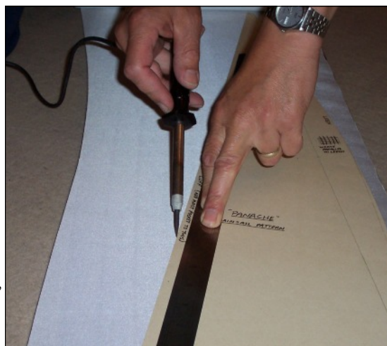
The new sails were cut out by running a pointed soldering iron bit round a thick paper template.
