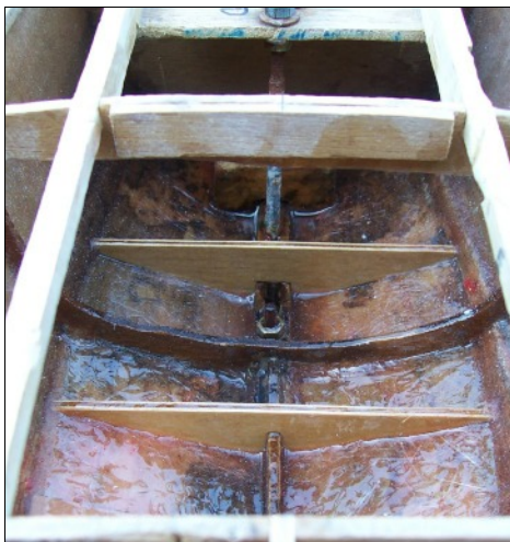
Half frames were inserted to stiffen the keel joint area and the inside of the hull was lined with fibreglass mat, tissue and resin to seal against water and stiffen it.
