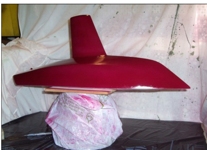
The hull after spray painting. The paint used was Humbrol Enamel diluted with cellulose thinners.
