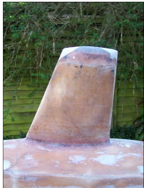
The hull/keel joint was reinforced and sealed with strips of fibreglass tissue and resin. The keel shape was also improved using car body filler.
