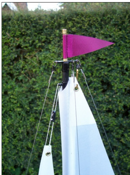
The new sails feature a pocket luff and ordinary dressmaking eyelets. Reinforcement in the corners is stuck on with double sided sticky tape. Most of the rigging is made from fishing tackle.
