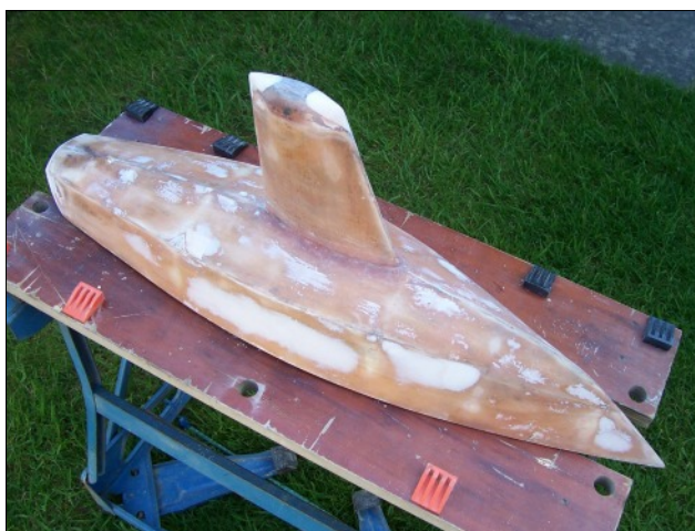
The hull showing all the areas filled with car body filler before spraying with yellow filler-primer.
