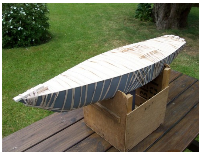
Gluing the new deck on with the help of 56 rubber bands and some balsa wood packing.
