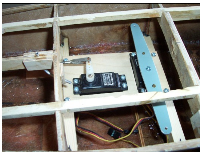
The radio gear was reinstalled on a plywood servo tray carried on softwood bearers across the hull. Short pieces of thin aluminium tube were fitted to carry the main sheet and jib sheet through the deck to the sail winch beam.
