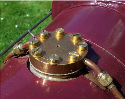
Top feed fitting on boiler. The red gasket sealer has all been cleaned off, 4BA screws fitted in place of the stripped 6BA items and a proper gasket fitted.
