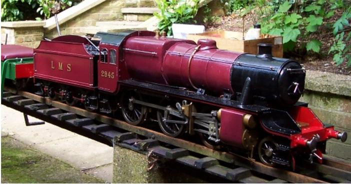
*This photo belies Princess Marina's dented boiler cladding and scruffy paintwork! However, she does have some nice detailing such as engine and tender brakes, hand-rails, dummy sand boxes and dummy steam pipes on the smokebox.*
