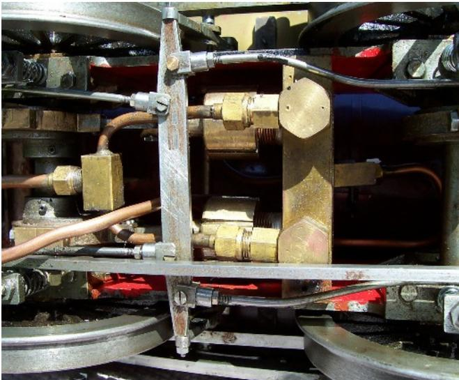
*Here you can see the twin axle driven pumps and split feed pipe hiding behind a brake beam. There was no packing in the pump glands! To the right of the pump body/frame stretcher block you can just see the pipe bracket whose fixing screw holes were drilled into the pump water passages.*
