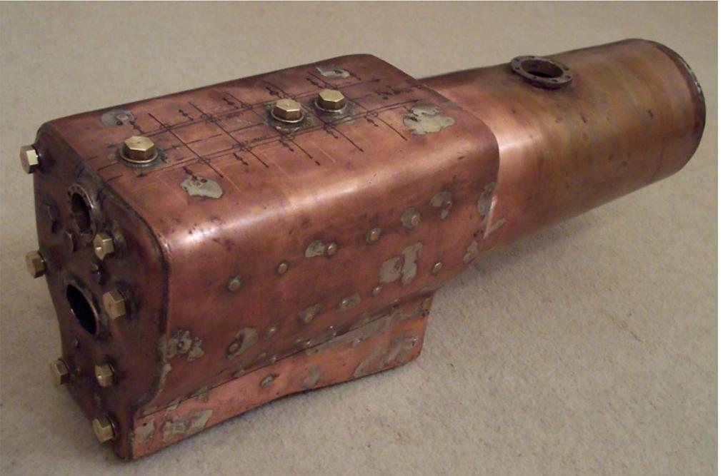
*My boiler after a good clean but before repair. The old regulator bush is still there but the positions of the rod stays have been drawn on the outer wrapper ready for drilling.*
