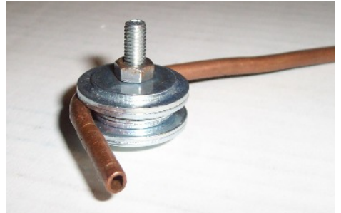
My home-made pipe bending jig made from a sandwich of 'repair washers'. Just anneal the copper tube, adjust the middle washers until it is a snug fit between the larger outer ones and pull it round with your fingers. Easy!
