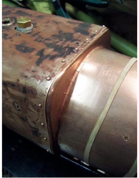
*Trial fitting of the cladding. The firebox cladding has been riveted to the transition piece and the barrel cladding sheet is held by elastic bands.*
