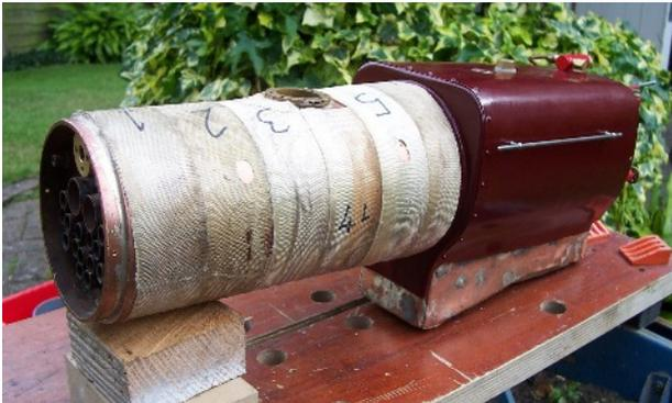
*The firebox cladding is in place over its lagging and the lagging is on the barrel. The strips of woven glass fibre tape were stuck together in a sheet using masking tape and then wrapped round the boiler.*
