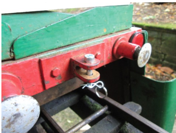
A typical coupling block. This one is on the rear of a passenger truck but it could equally be on the back of your loco.
