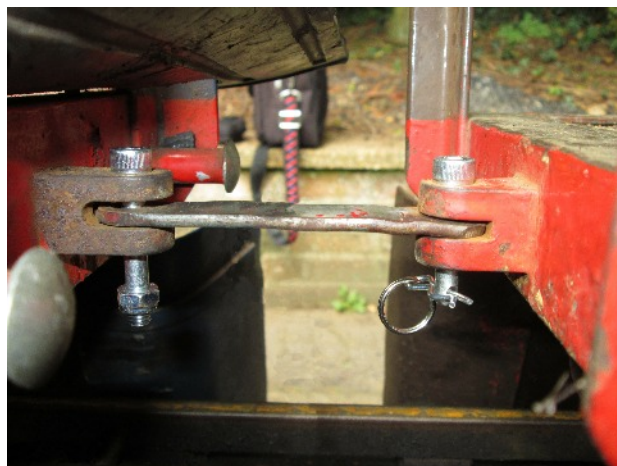
A typical bar coupling. The bar is held in the coupling blocks by pins which are retained by an 'R' clip (right) and a Nyloc nut (left).
