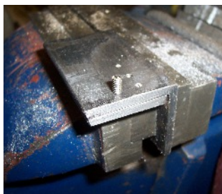
2. Clamp the jig in a bench vice with the excess screw end sticking upwards.
