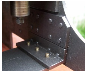
The frame extension joint with the screws shortened. That looks better!
