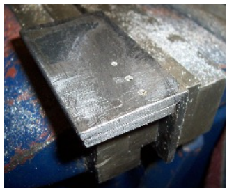
4. Remove the remaining excess with a fine file leaving the screw flush with the jig.
