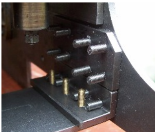
This was my frame extension joint with 1/2" 5BA screws fitted. They are a bit long.
