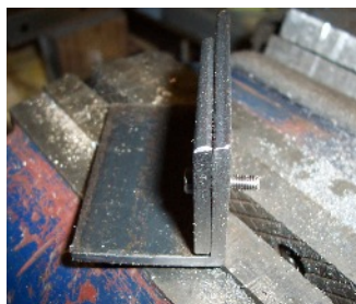
1. Put the screw in the jig with the amount you want to cut off sticking out.
