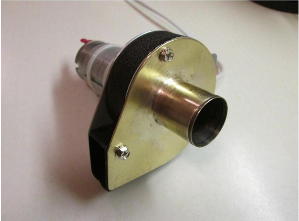
*Here is the finished item after re-heating with salty flux! There is now a nice neat fillet of solder all round the base of the tube.*
