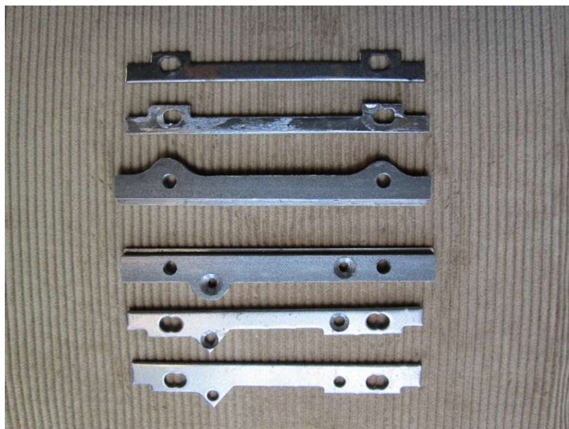
The reverse side of the original door runner components and the new one piece runners. The rebates in the new runners that the doors slide in can be seen clearly.
