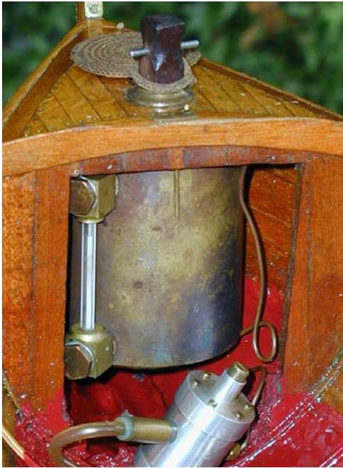
Gas tank and regulator installation. Note the level glass.
