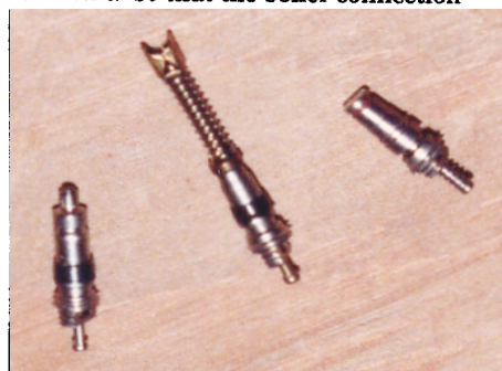
Three common types of car valve. Left hand one is the design required for the gas controller.
