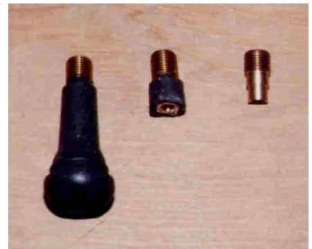
Modification to the car type valve holder. The holder is gripped for machining in a split collet threaded \frac{1}{16} in. \times 32tpi.
