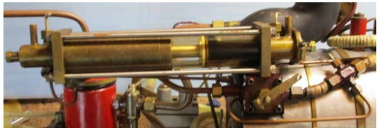
is isolated from the boiler pressure and oil is pumped in through the vertical pipe at the oil end, pushing the piston back and emptying condensate from the steam end. It was all made this way so that the oil could be replenished with the boiler at full pressure. In fact the lubricator allows several hours running before it has to be refilled.
