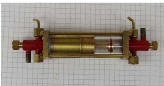
Also pictured here is a much smaller version (photographed on 1/8" graph paper) which has the large bore of 1/2" and the smaller of 8mm.
