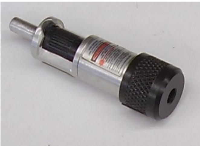
Laser alignment tool – invaluable on the milling machine, very quick and easy to use.
