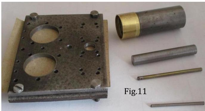
The punch consists of two 1/8” steel plates with all the round holes needed for the two designs. There are four different diameters needed, the smallest just acting as the corners of other cut outs. Figs 11,12 & 13 show the punch plates and punches; gaskets as they come out and cut outs; and the finished gaskets.
